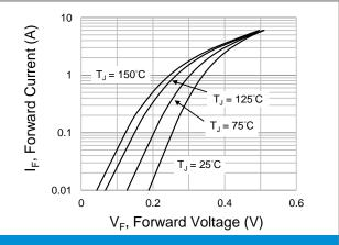
**Fig.4 Typical Forward Characteristics**
