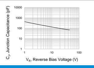
**Fig.2 Typical Junction Capacitance**
