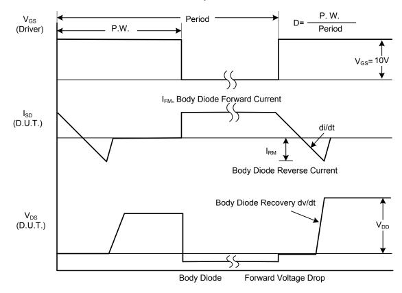
Peak Diode Recovery dv/dt Waveforms
